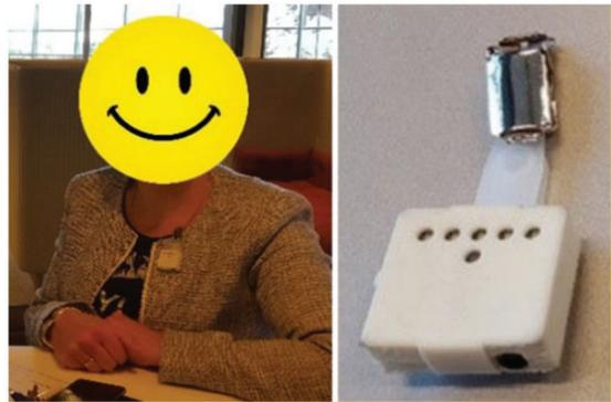
**Figure 2** Participant wearing a Lightlog (left) and separate picture of the Lightlog wearable photometer developed by Martin (right).<sup>39</sup>
