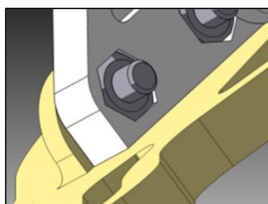
Figure 10-3: Locked nut - detail view
