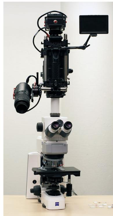
Fig. 2. The RED ONE video camera connected to the microscope.
