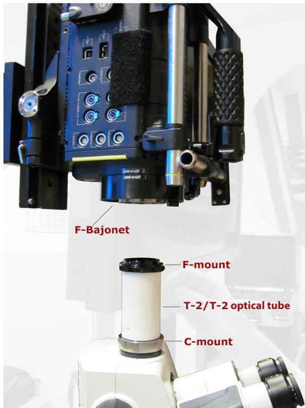
Fig. 3. Optical tube with F-mount and C-mount; the RED ONE video camera with the Nikon F-bajonet.
