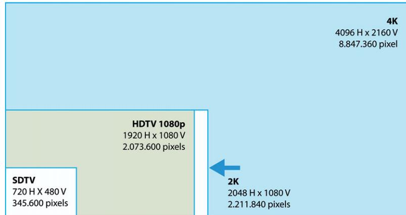
Fig. 1. 4K resolution in comparison to other resolutions.
