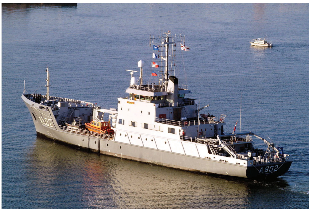
Figure 4. HNLMS Snellius, hydrographic survey vessel (length: 82 m, beam: 13.1 m, draught: 4 m, displacement: 1875 tons, speed: 12 kts, built: 2003, propulsion: diesel-electric 1250 kW, crew: 18)
