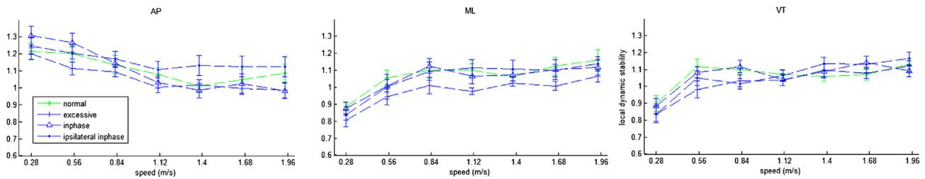
**Fig. 2.** Dynamic stability quantified as the group-averaged short-term local divergence exponent ( $\lambda_s$ ). The left panel presents  $\lambda_s$  for the AP direction, the mid panel for the ML direction and the right panel for the VT direction. Each panel presents all arm swing instructions, see legend in the left panel, and all gait speed conditions. Error bars present the standard error.
