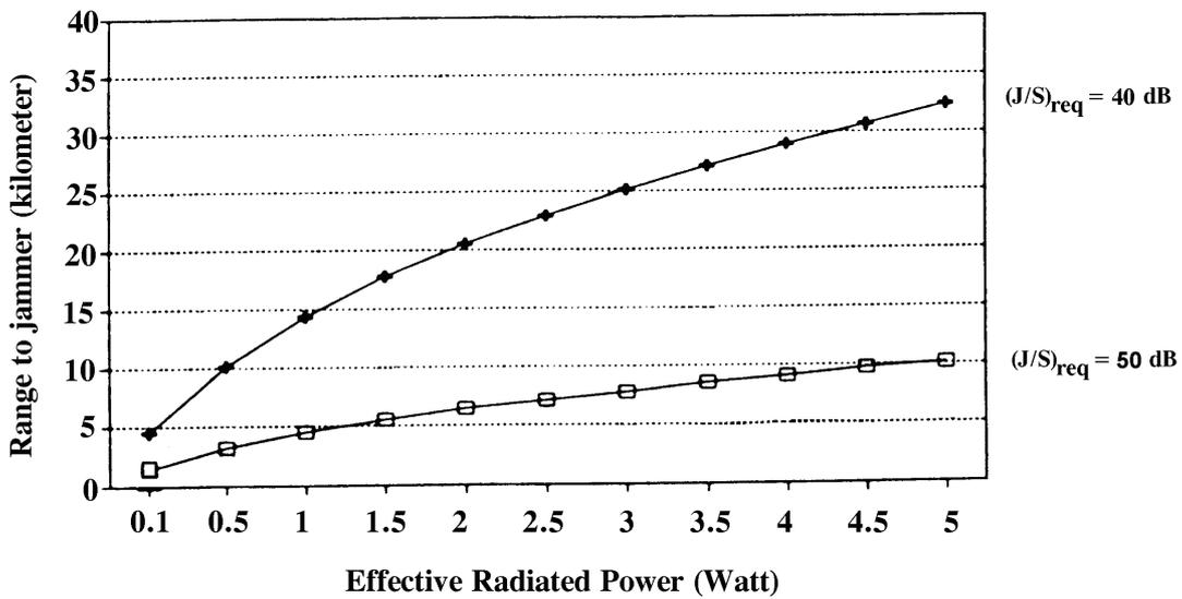
Figure 10: Dependence of the effective jamming range on the radiated power of the jammer
