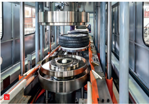
2 Examples of complex products that required multidisciplinary engineering from RAAK-MKB participants. (a) Palletizer (CSi Industries). (b) Robot food packaging handler (LAN Handling Systems). (c) Bead optimisation system (Fontijne Grotnes); the bead is the edge of a tire that sits on the wheel.
