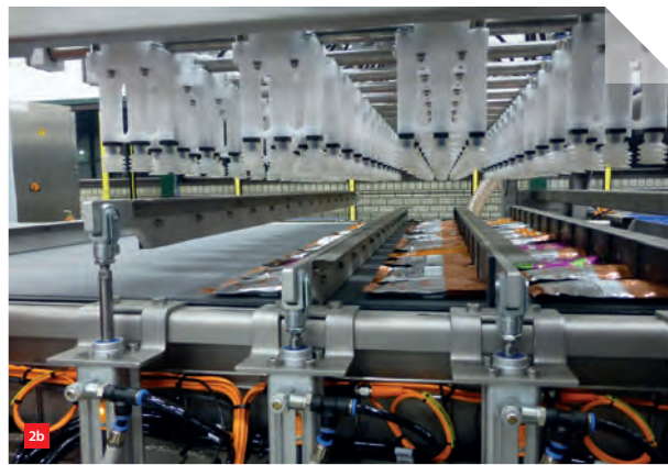
2 Examples of complex products that required multidisciplinary engineering from RAAK-MKB participants. (a) Palletizer (CSi Industries). (b) Robot food packaging handler (LAN Handling Systems). (c) Bead optimisation system (Fontijne Grotnes); the bead is the edge of a tire that sits on the wheel.
