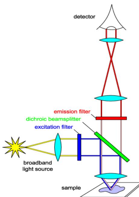
Figure 9. A simplified illustration of the principle of a fluorescence detector [22].
