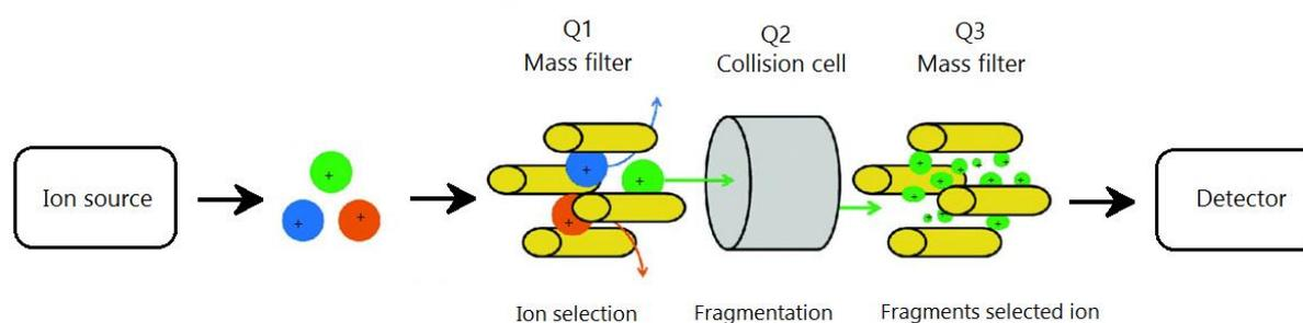
Figure 11. A representation of a triple quadrupole mass spectrometer using product ion scan mode.
