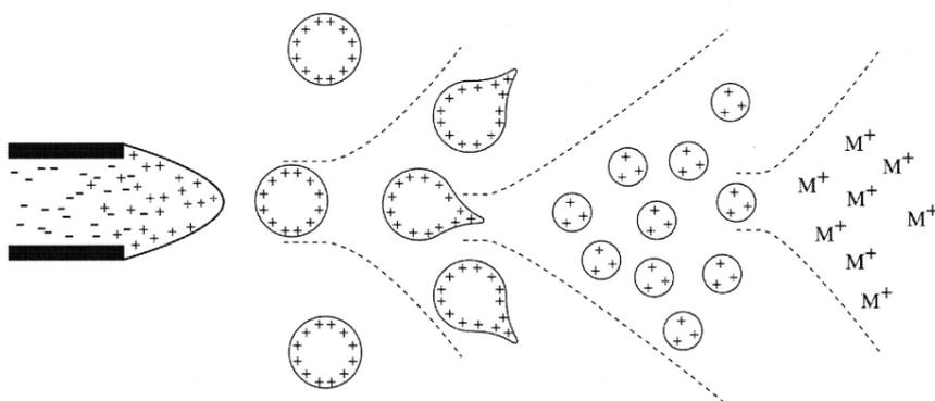
Figure 10. Mechanism of electrospray ionization [23].
