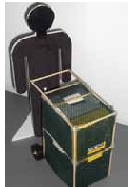
Figure 6. A scale-model of the converter unit design, now with wheels for easier transport. Both size and weight actually turned out larger than those of the mock-up.
