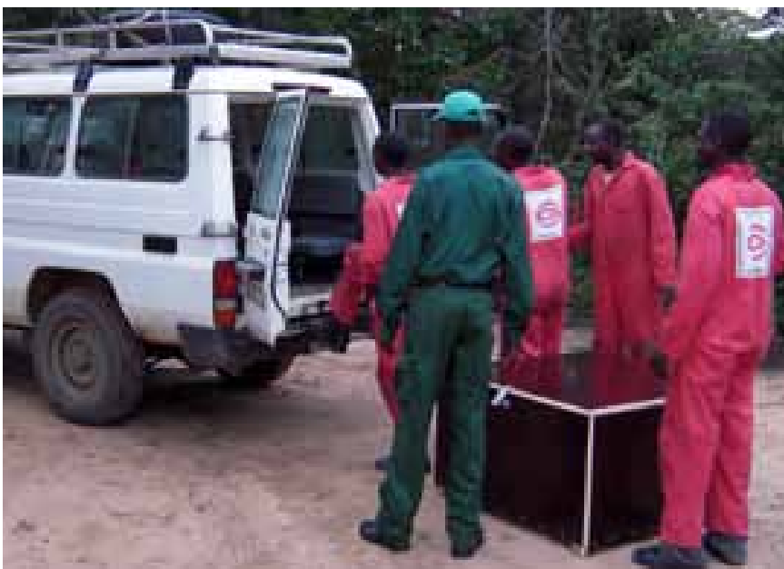
Figure 5. Angolan deminers test the handling of a mock-up of the converter unit, at a time when measurements were yet unknown. The mock-up was simply an empty plywood box 100 x 100 x 50 cm containing batteries for weight. Based on this experience, all agreed that this size was far too big for easy handling.
